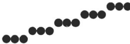
Figure 3-1 Stairstep effect (jaggies) produced when a line is generated as a series of pixel positions.
